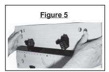
Step 3) The Swivel Pegs (#1) and Peg Supports (#5) can be placed into any hole in the Work Table top provide a block to secure and block your workpiece.
